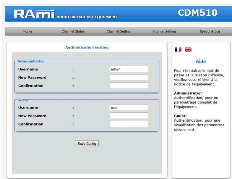
User and password configuration page. Required to access the device configuration pages.
