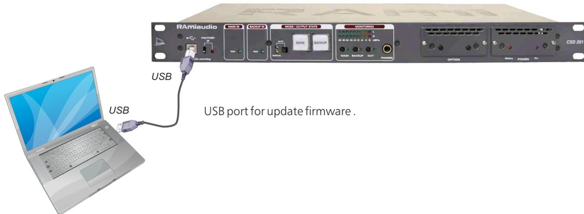
**- Step 2 :** CSS201 has been recognized by your computer. It is now necessary to load the new firmware with the supplied software "Rami-AMIX Firmware Updater". To do this, open the supplied software and then the program "Hex" file.
