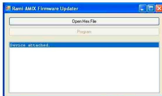
**- Step 3 :** This last step allows you to flash CSS201. To do this, click on the "Program" button of the supplied software "Rami-AMIX Firmware Updater". Once programming is complete, you can disconnect the USB cable from the device.
