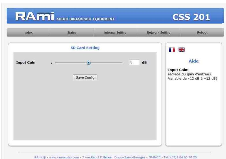
**Input Gain:** setting the input level of the SD card. Variable from -12dB to + 12dB.
