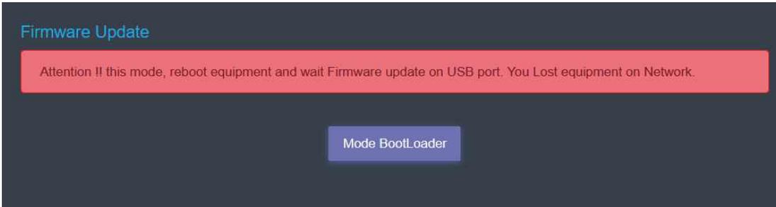
**Warning:** This mode reboots the device while it is waiting for an update via its USB port. The IP connection is disabled during this update.
