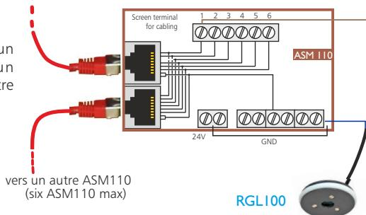
RGL100 is a light indicator, used to show the "ON AIR" microphones in a broadcasting environment. It fits easily between the microphone holder, and the microphone support. Use of led results in a very long life.
