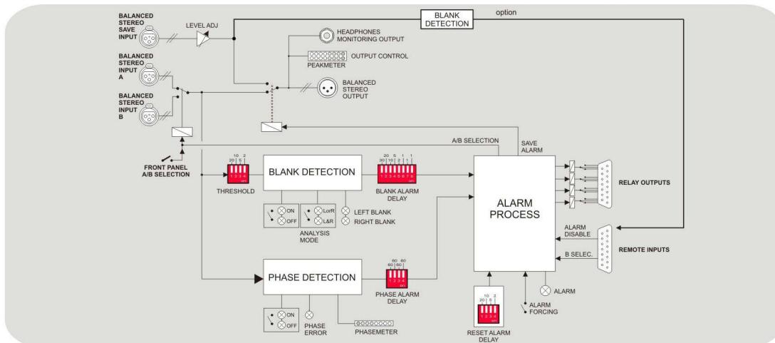
**CSS 203** would be used in radio broadcasting stations, for example, as a backup to the broadcast in case of main modulation disconnection. It would preferably be situated at the end of a broadcasting installation or just after the satellite receiver for regional disconnection in local stations.
